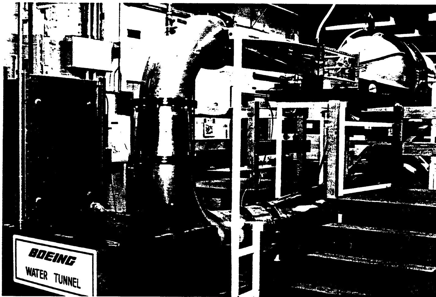
4.5-inch by 12-inch water tunnel.
